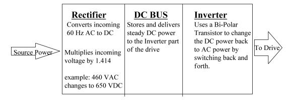
The components of the drive system are broken into four major categories: Source power, VFD, Cable and the Motor. Other ancillary components exist such as resolver and encoder feedback devices, tachometers, sensors, relays and others that help supplement the system.
