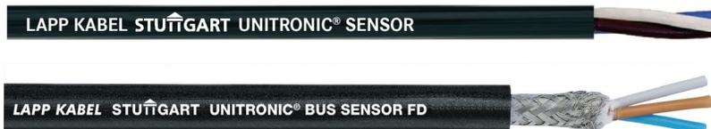
UNITRONIC® SENSOR FD is designed for sensor and actuator wiring. Constructed with extra-fine stranding, this cable is suitable for continuous flex applications. The abrasion- and tear-resistant PUR jacket provides superior service life in harsh environments and is also resistant to most oils, solvents, and coolants.
