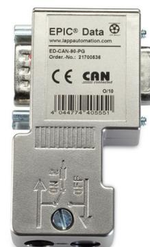
EPIC® Data CAN bus connectors are screw terminal, 9 pin D-Sub connectors with an integrated adjustable termination resistor. The cable entry is 90° angled. Connectors are available with additional programming/diagnostic interface.
