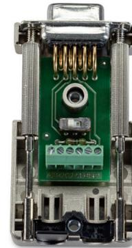
EPIC® Data CAN bus connectors are screw terminal, 9 pin D-Sub connectors with an integrated adjustable termination resistor. The cable entry is 180°. Connectors are available with additional programming/diagnostic interface.
