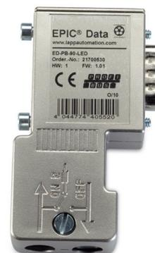
EPIC® Data PROFIBUS connectors are screw terminal, 9 pin D-Sub connectors with an integrated adjustable termination resistor. The cable entry is 90° angled. Connectors are available with additional programming/ diagnostic interface.
