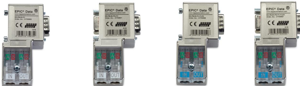
EPIC® Data PROFIBUS connectors are fast connect, 9 pin D-Sub connector with an integrated adjustable termination resistor. The cable entry is 90° angled. Connectors are available with additional programming/diagnostic interface.
