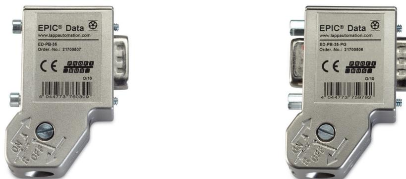
EPIC® Data PROFIBUS connectors are screw terminal, 9 pin D-Sub connectors with an integrated adjustable termination resistor. The cable entry is 35° angled. Connectors are available with additional programming /diagnostic interface.
