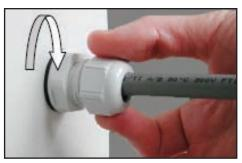
4. Tighten the cap nut by hand with a clockwise rotation while holding the pressure nut.
