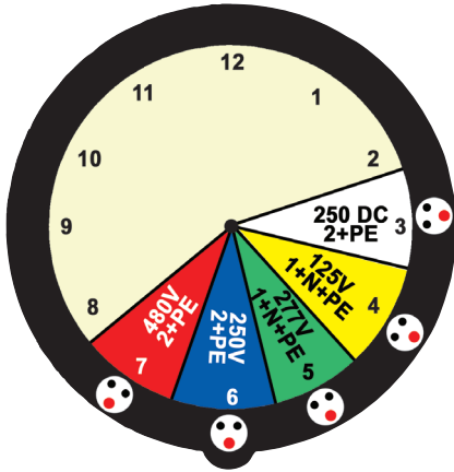
3 Wires: 2+PE & 1+N+PE
