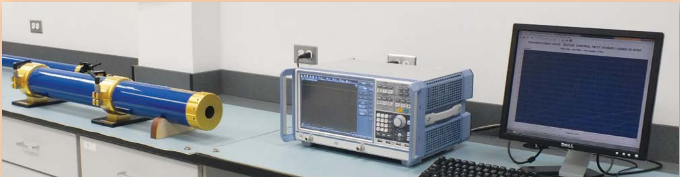
The test Equipment Lapp USA uses are a network analyzer and a precision tube to measure the transfer impedance of a shielded cable. The transfer Impedance test is performed per EN 50289-1-6 / IEC 62153-4-3 Ed2 Surface Transfer Impedance – Triaxial Method. The test setup consists of a network analyzer and a precision tube with terminations to the cable screen and the network analyzer.
