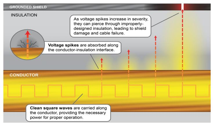
There are many methods of diminishing unwanted electrical conditions in the components of a VFD system. In order to protect cables from power distortions during the process of rectification, the 2020 National Electrical Code requires that the size of source power conductors is 125% of the full load current of the drive. Changing the pulse rate or switching the inverter to a slower frequency can eliminate some harmonics.
