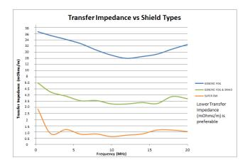
Note: Transfer Impedance relates to a current on one surface of a shield to the voltage drop generated by this current on the opposite surface of the shield. Transfer impedance is used to determine shield effectiveness against both internal and external interference signals. Higher transfer impedance values are indicators of poor performance of the overall cable shield.
