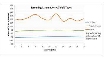
Note: Screening attenuation is the measurement of decibel ratio between the internal and external signals of a device. In short, it is a ratio of electric or magnetic field strength before and after placement of a shield. For Screening Attenuation readings of lower dBs are indicators of poorer overall shield effectiveness performance.
