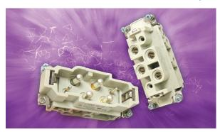
EPIC® Power K series inserts provide a combination of power contacts (up to 80A) and signal contacts (up to 16A) in a single insert package. This can save valuable panel space by allowing one connector to do the job of two. These inserts fit into EPIC® HB series housings.
