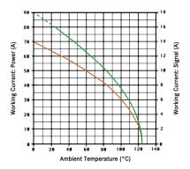
EPIC® Power K 4/8 6 AWG (16 mm<sup>2</sup>) power 14 AWG (2.5 mm<sup>2</sup>) signal
