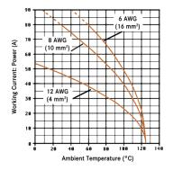
EPIC® Power K 4/2 12 AWG (4 mm<sup>2</sup>) power 18 AWG (1 mm<sup>2</sup>) signal
