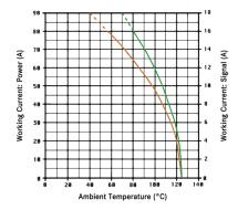
EPIC® Power K 4/8 10 AWG (6 mm<sup>2</sup>) power 18 AWG (1 mm<sup>2</sup>) signal
